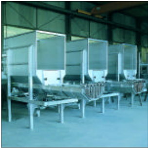
Figure 36 Trough feeders in a canning works; the troughs and hopper walls coming in contact with the product are made of textured plate to prevent the wet slices of vegetables from clinging
