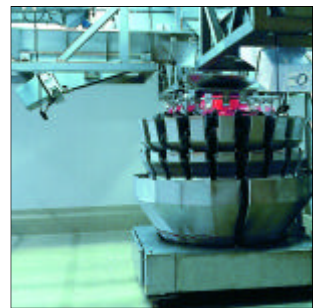
Figure 8 Electromagnetic vibrators of the MX series can be easily controlled during operation, and stop immediately when switched off. They are therefore suitable as drives for bin discharge conveyors and scales loading.
