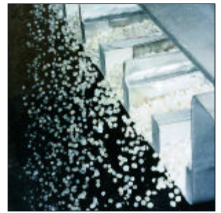
Figure 14 Numerous tasks sprinkling onto mats, belts, dough etc. can be handled with vibratory conveyors
