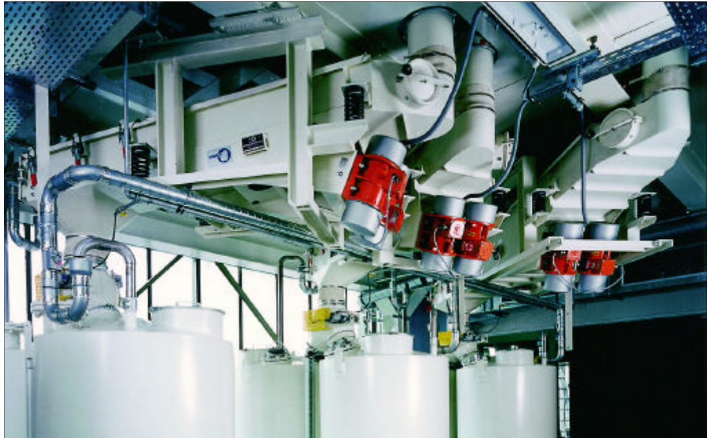
Figure 37 Vibratory conveyors in a chemical factory fitted underneath the ceiling
