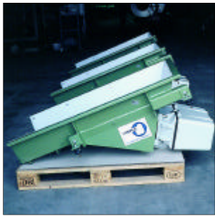
Figure 23 Bin discharge vibratory con- veyors with wear lining
