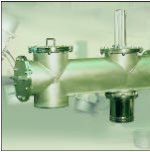
Figure 9 Specially constructed intermediate outlet with pneumatically operated cone stopper
