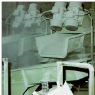
Figure 15 The vibratory drives are also suitable for application into tough and dusty environments
