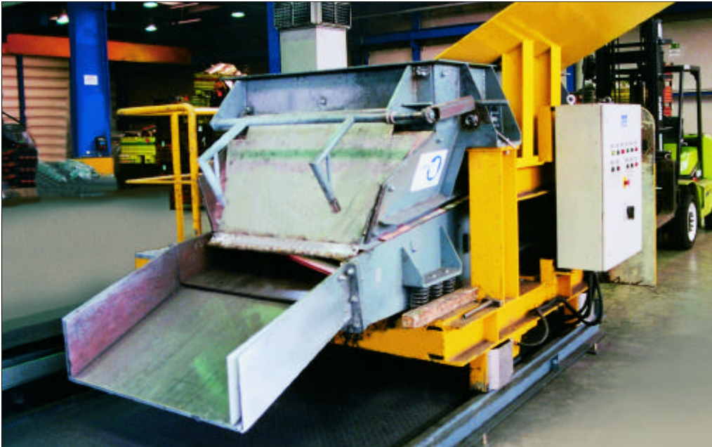
Figure 39 Mobile furnace charging equipment for feeding brass scrap to a melting furnace
