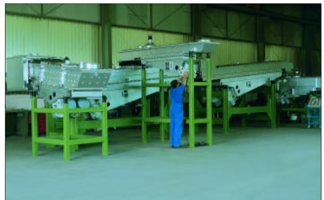
Figure 13 Vibratory conveyors for cooling ash and bed material 400-800 °C
