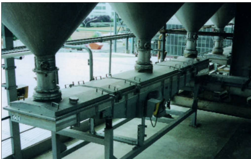
Figure 7: Vibratory trough conveyors 800 mm wide, 6.5 m long, used as bin discharging conveyors in a chemical factory
