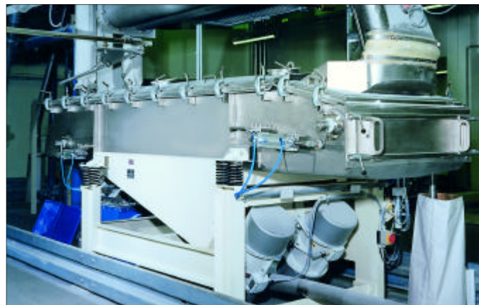
Figure 33 Vibratory trough conveyors with integrated screen decks have the advantage of low height. The figure shows a single deck machine with pneumatically operated screen tensioning in a foodstuffs factory.
